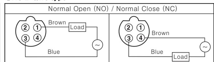
※In case of AC switching type, ② and ③, ① and ④ are connected to each other inside.
