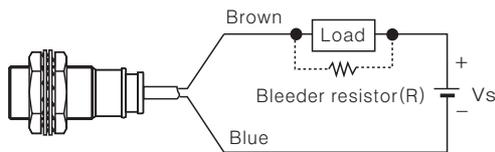
Please make the current on proximity sensor smaller than the return current of load by connecting a bleeder resistor in parallel.
