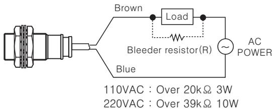
It may cause return failure of load by residual voltage.
