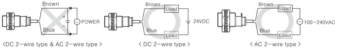
When using DC or AC 2-wire type proximity sensor, the load must be connected otherwise internal components may be damaged. And the load can be connected to either wire.
