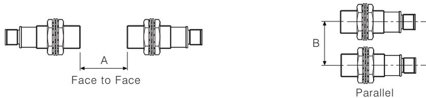
When sensors are mounted on metallic panel, it must be prevented sensors from being affected by any metallic object except target. Therefore, be sure to provide a minimum distance as below chart.
